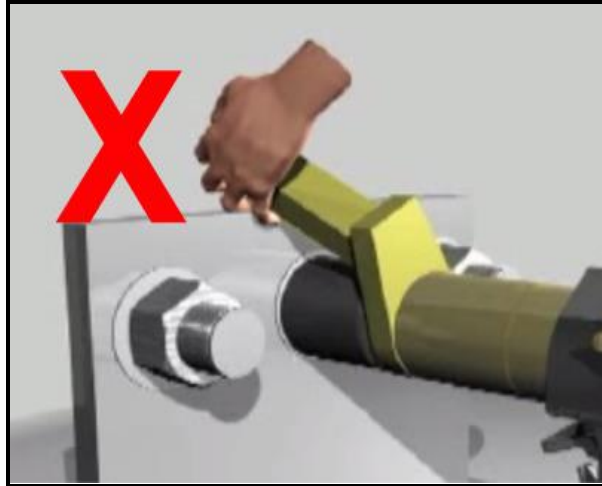
Figure 5.1.1-2: Incorrect Placement of Hand/Body Parts During Operation
